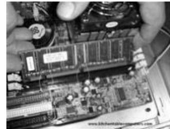
Once you're sure you have the right RAM, to actually insert it, simply push it firmly, straight down into the slot, and push the retainer clips inward. That's it.
