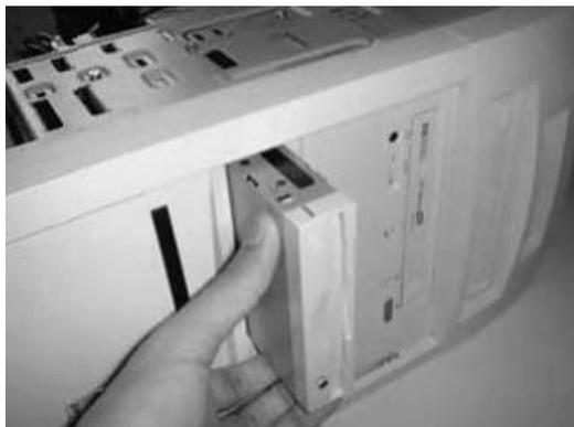
Place the ZIP drive into a mounting slot and screw it securely into position.
