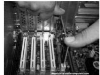
You may have to use some oomph here. If the card doesn't seat itself using fingertip pressure, place your palm over the card and push down firmly and evenly until you feel the card pop into place. But first check the slots, notches, and tabs to make sure you're not trying to install the card in the wrong slot.
