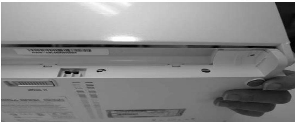
Fasten all 9 Phillips-head screws. Failure to apply any screws will damage the notebook.
