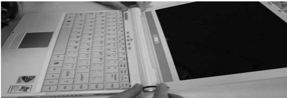
Hold the hinge cover and snap it in place. Push downward at each end of the cover to secure it.
