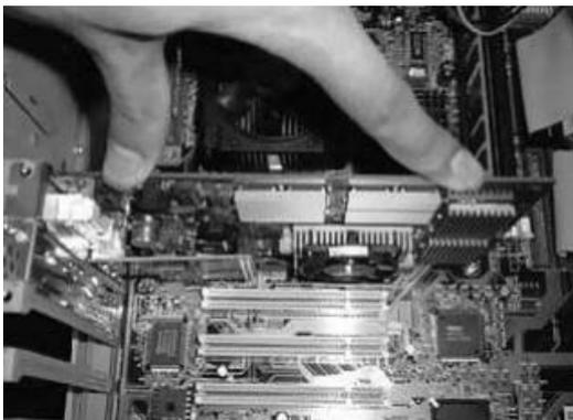
All you need to do now is to screw the metal plate on the front of the card to the ATX case. Use the screws supplied with case and screw the card to the case.
