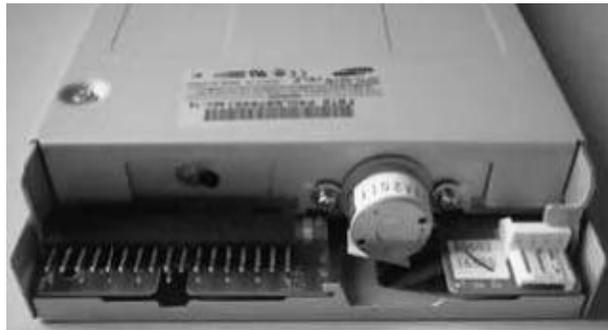
The black connector on the left hand side is the floppy disk connector. It is different from the IDE connector and uses a different cable. The small white connector on the right hand side is the power connector for the floppy drive. Figure 1 and 2 below shows what a floppy drive cable and floppy drive power connector looks like.
