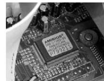
BIOS its name. They manage things like the keyboard, the screen, and the serial and parallel ports, especially when the computer is booting.
