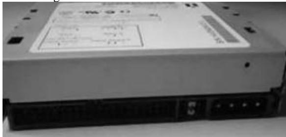
On the left hand side you have the IDE connector. On the right hand side you have the power connector. In the middle you have the jumpers. You have to specify if the ZIP drive is being connected as a Master or a Slave device using the appropriate jumper setting.
