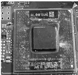
soldering. Surface mounting the CPU saves the laptop manufacturer money and time in production. The main reason for socketing laptop CPU's is probably to allow for last-minute changes in market targeting as CPU prices comes down and the competition heats up.
