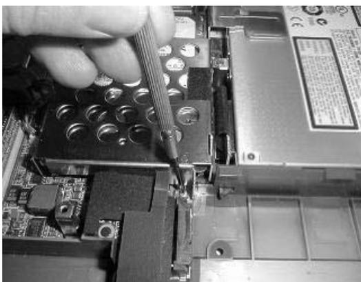
to. OK, I got my hand in the way a little here, but there's a standard 2.5" laptop hard drive in the metal cage with all the round holes in it. The cage is held in place with three screws, the first of which I'm taking out. To the right is the DVD drive, and if we were replacing the DVD, the single screw on the tab to the right of the hard drive is all that's holding it in place.
