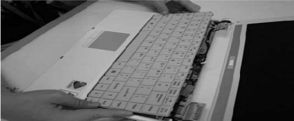
Connect the cable underneath the hinge cover. There is only 1 correct connection of connecting the cable. Be careful not to damage the antenna PCA that is connected to the left and right display assembly hinges. Damaging either antenna PCA can degrade notebook performance.
