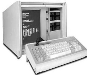
In February 1984, IBM announced the IBM 5155 Portable Personal Computer (laptop, notebook). This Portable PC was IBM's first carry around computer. It required AC power to be plugged in to work and weighed 13.6Kgs. IBM would cease manufacturing the 5155 laptop in April 1986.
