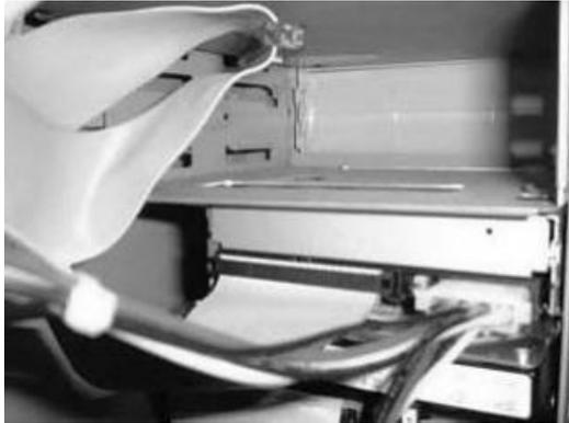
Connect the power cable and the IDE cable to the corresponding connectors. Connect the other end of the IDE cable to the IDE socket on the motherboard. Make sure the pin 1 on the cable connects to pin 1 on the motherboard IDE socket and on the ZIP drive socket. The rear end of your CD-RW drive should look similar to the image below.
