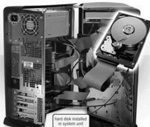
Figure: A hard disk is enclosed inside an airtight, sealed case inside the system unit
