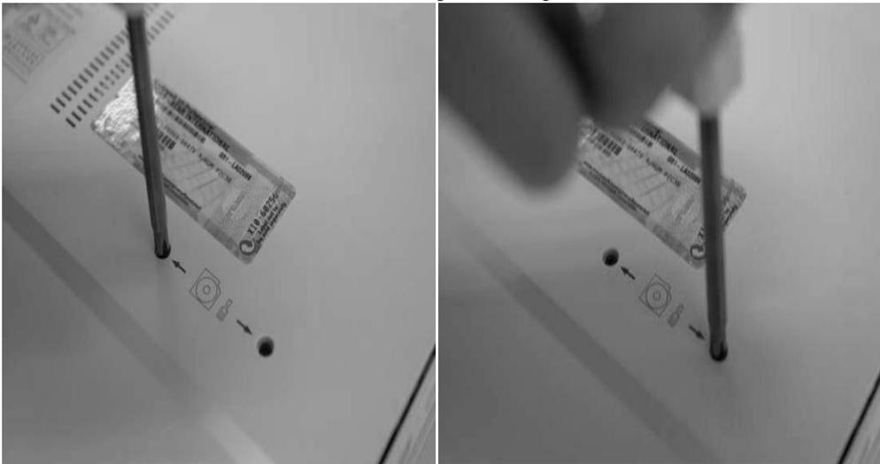
Pull out the optical storage device from the notebook, then insert the new optical storage device.
