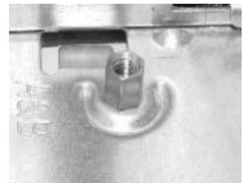
Standoffs must NEVER be inserted into any of the "extra" holes, however. Standoffs installed in holes on the case that don't have corresponding holes in the motherboard can cause the motherboard to short out.
