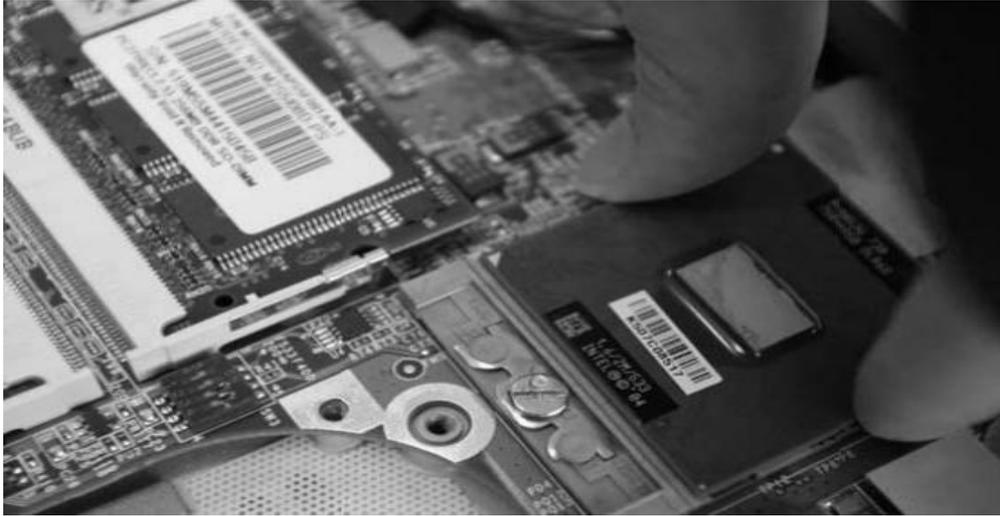
You do not have to press down the processor. If the processor does not drop completely into the socket, turn the actuator until the processor drops in completely.
