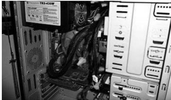
A typical installation of an ATX form factor computer power supply.
