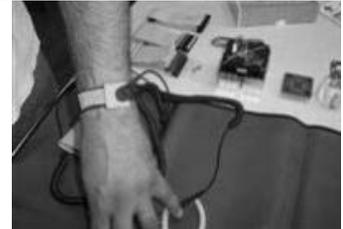
The wrist strap attaches to the computer's chassis by means of a high-tech device commonly known as an alligator clip. Connect the alligator clip to an unpainted, metal part of the computer chassis, and check it frequently to make sure it hasn't fallen off.
