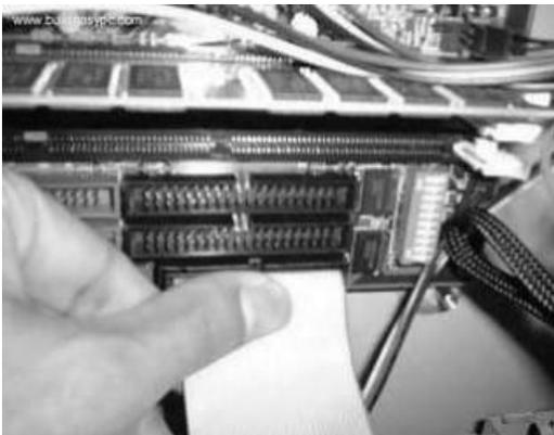
Finally connect the other end of the floppy drive cable to floppy drive connector on your motherboard. Make sure pin 1 on the cable connects to pin 1 on the connector. If you look at the rear side of your CD / DVD-ROM it should look similar.
