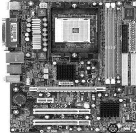
An alternative way to clear the CMOS is by removing the CMOS battery with the system unplugged for about ten minutes. The CMOS battery is round and silver, and is retained by a small clip. Be careful when you place it again in its position, to seat it with the correct polarity up:
