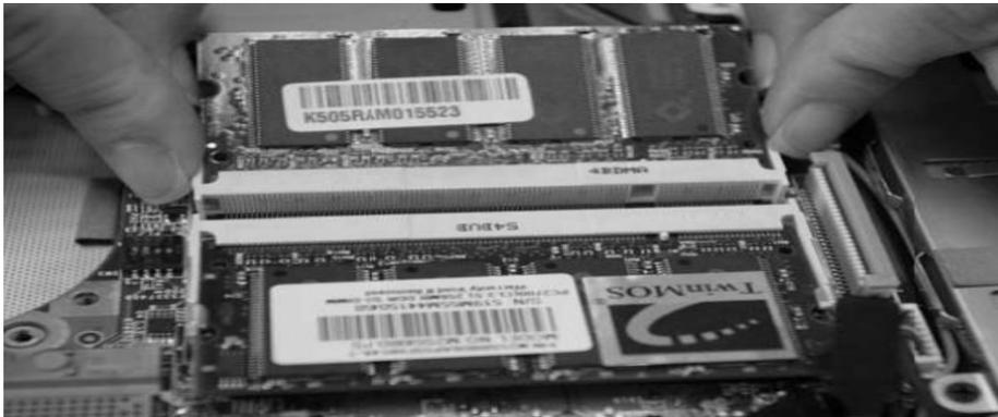
If you have more than one memory module, please align the 2nd memory module to the DIMM socket 2. Memory should be inserted firmly at a 45 degree angle and pushed down until module snaps into place. Memory module can only fit in one direction due to the keyed notch. Wrong orientation will cause improper installation and may damage the memory modules or DIMM soc.
