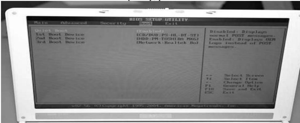
Insert a bootable OS C D into the OSD tray. To save/exit the BIOS Setup Screen, press “Y” to save/exit.
