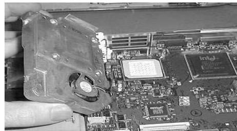
There's no space between the substrate and the motherboard for pins, it's a BGA (Ball Grid Array). Some super ambitious do-it-yourselfers might try to desolder the CPU with a hot air gun, and it might work to remove it, but I wouldn't give good odds for getting a replacement CPU to operate with
