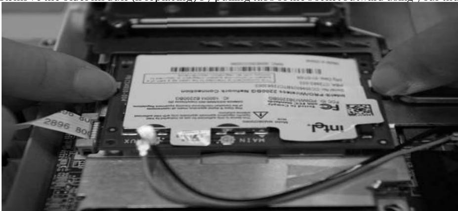
The module should pop up into a 45 degree angle. Remove the module by pulling it gently backward. Use side-to-side motion, if necessary, to remove. Unplug the antennas. Mini PCI module should be inserted firmly at a 45 degree angle and pushed down until module snaps into place. After the module snaps into place, connect antennas on the Mini PCI module.
