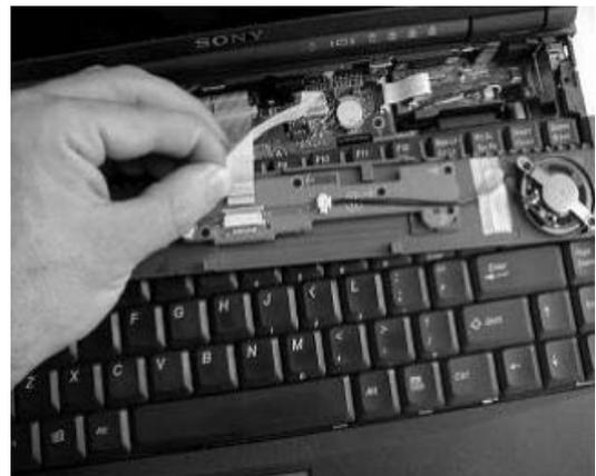
The inside of the Sony notebook computer body. The ribbon cable that powers the speakers is removed above, simply by pushing back the edges of the white connector, then pulling out the ribbon. There's a similar connector on the back of the keyboard, which we lift out to the left, giving us access
