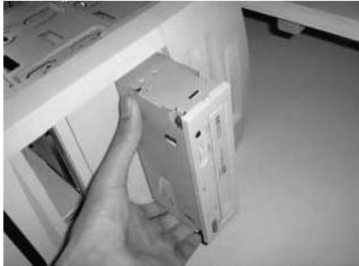
Connect the IDE and the power cable to the drive. If you want to use the CD-RW drive for playing Audio CD's then you also need to connect an audio cable to the Audio-out socket of the drive. If you have a CD/DVD-ROM then the audio cable is usually connected that drive instead of the CD-RW, but there is no reason why you can't have both.
